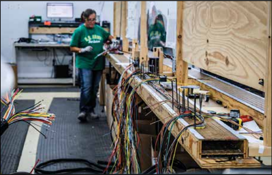
Harness layout boards using the pegboard method.
