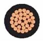
Once the wire is inserted into the terminal block, and the cage closes and clamps on to a tinned wire, the tin/wire block is compressed and can change shape. In doing so, the tin can fracture and cause wire strands to pull apart from one another, creating voids (Fig. 1). Essentially, as the wire is screwed down, it breaks apart the tin, which can start to loosen the wire. While the wire may be secure
