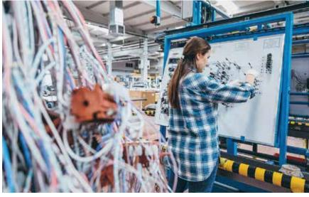
Preassembled harness, automating part of the assembly process.
