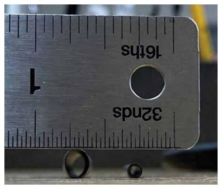
Figure 1: The figure shows the cross-section of a sample of heat shrink tubing both before and after unrestricted shrinkage. To verify the dimensional life of the sample at any time, a measurement of inner diameter is recorded followed by unrestricted oven shrinkage of the sample. After the shrinkage, the inner diameter is re-measured and the wall thickness is measured.
