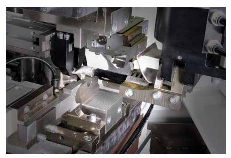
Smart robot feeding of loose terminals on the Artos CrX-44HD.
