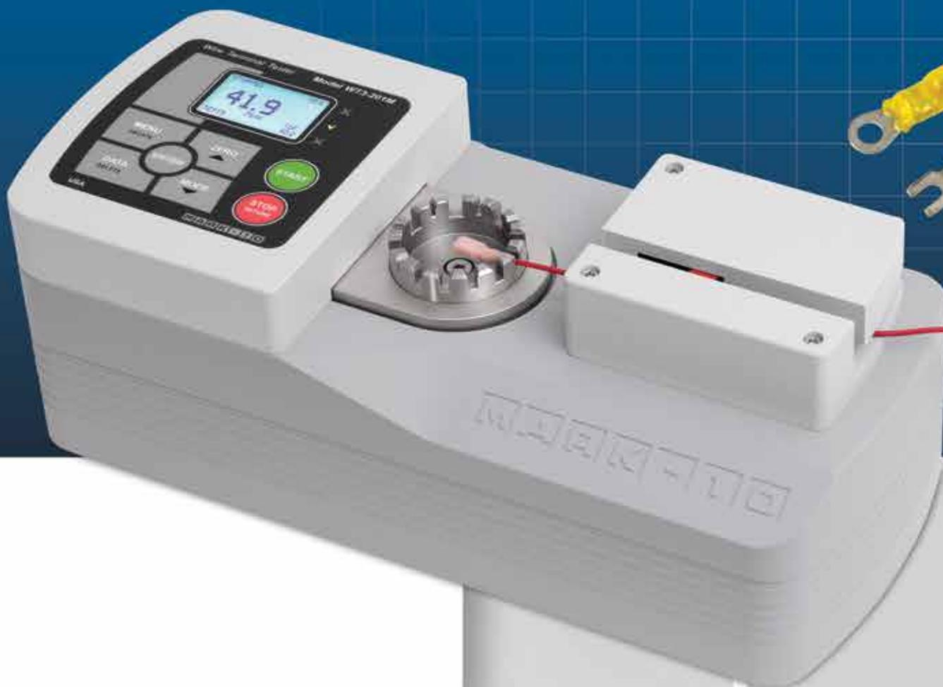
Whether pulling to a break, pulling to a force, or holding at a force, rely on Mark-10 pull testers to satisfy your UL, ISO, ASTM, SAE, MIL, and other testing requirements up to 1,500 lbF / 6.7 kN of force.
