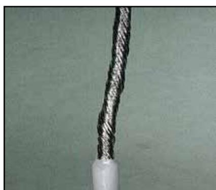
Figure 10. Overtwisted wire.
