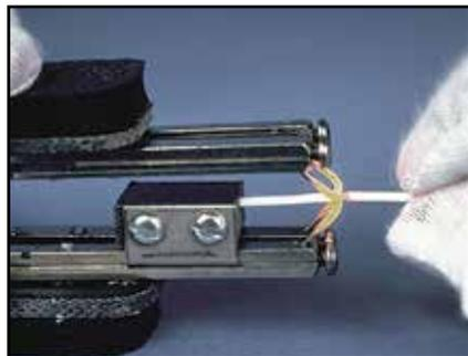
Figure 7. Melt through insulation.
