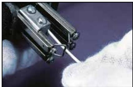
Figure 6. Firm insulation contact.
