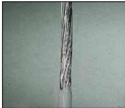
Figure 9. Birdcaging of straightened wire.
