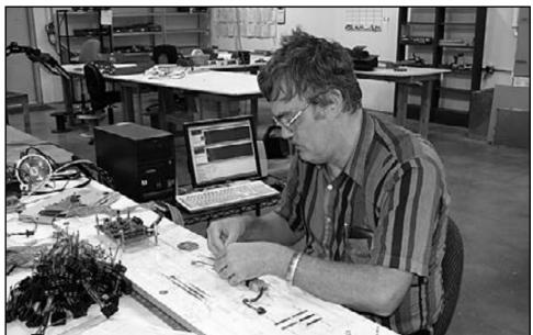
Robert Cashatt performs 100% QC test on a wire harness using an assembly test fixture and Cable Eye Cami M3 circuit tester.
