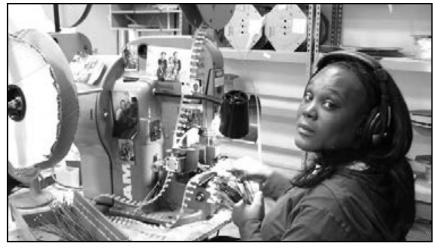
Tashia Taylor uses one of six crimping presses to apply terminals to wires.
