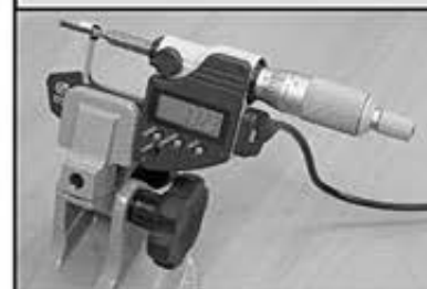
Measure conductor and insulation crimp heights
