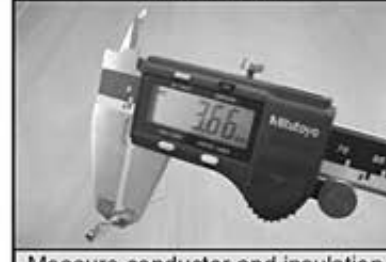
Measure conductor and insulation crimp widths
