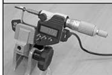
Measure conductor and insulation crimp heights
