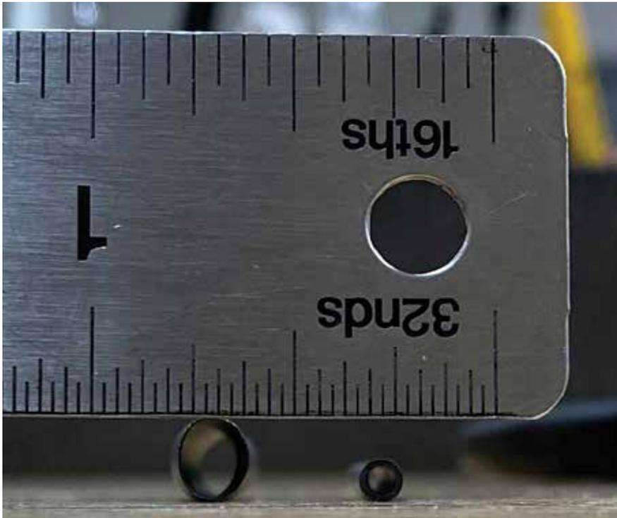
**Figure 1:** The figure shows the cross-section of a sample of heat shrink tubing both before and after unrestricted shrinkage. To verify the dimensional life of the sample at any time, a measurement of inner diameter is recorded followed by unrestricted oven shrinkage of the sample. After the shrinkage, the inner diameter is re-measured and the wall thickness is measured.
