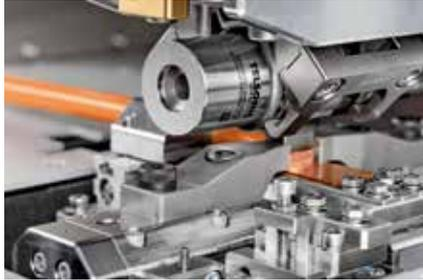
Following are some specific applications and challenges for ultrasonic welding of stranded wire on terminals:
