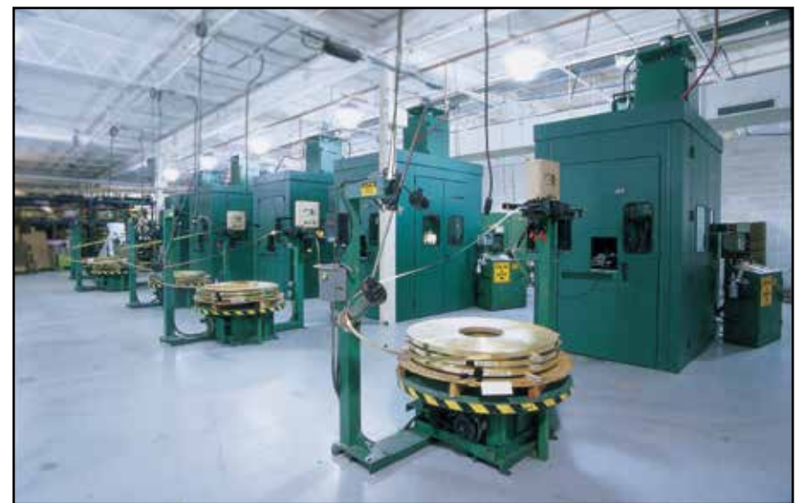
Bruderer presses enclosed in sound deadening boxes.
