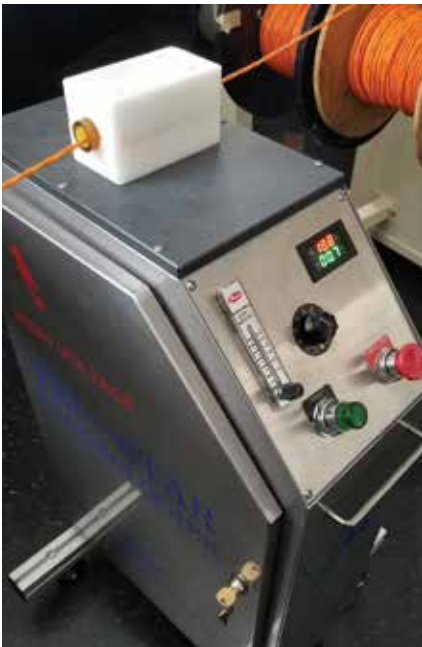
Figure 2. Wire fed through plasma chamber.
