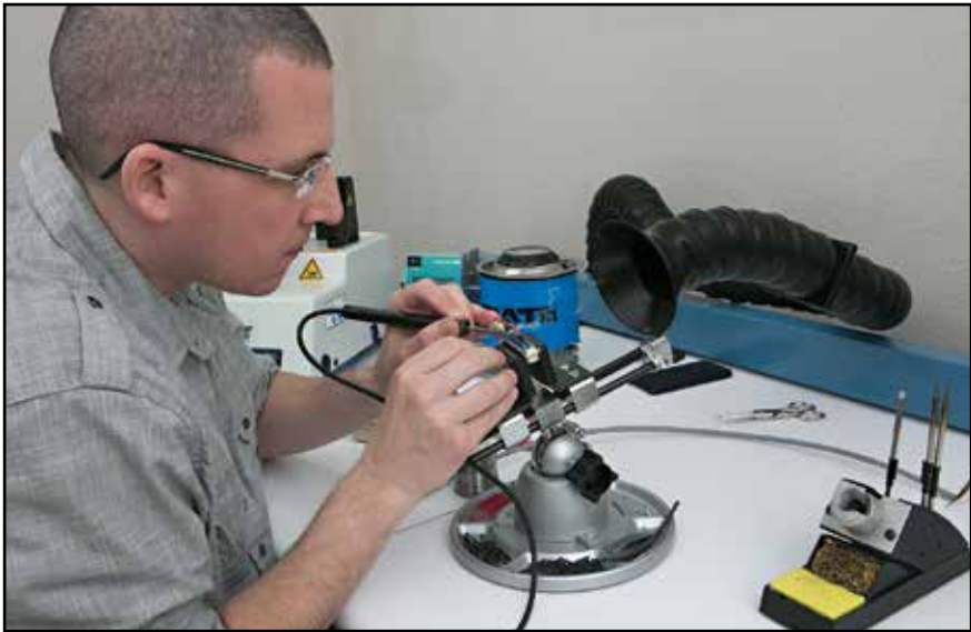
Northcomm tries to avoid manual assembly processes, but some products require careful hand soldering.
