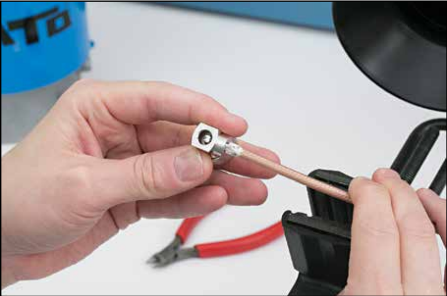
Inspection of Amphenol RF right angle connectors on RG-400 cable assembly.
