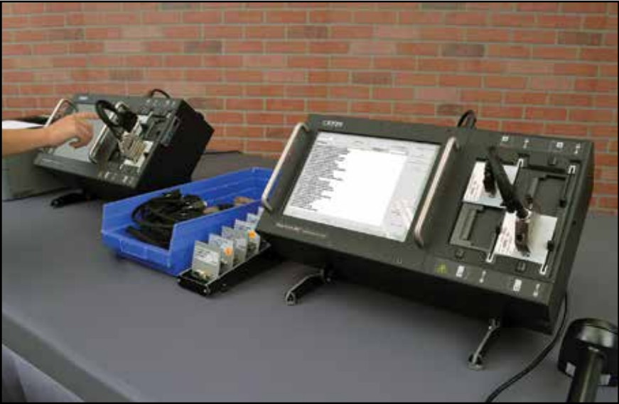
Figure 1. Testers with interchangeable adapter boards for easy switch over between cables. (Photo Courtesy of Cirris)
