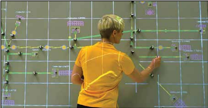
Wire harness assembly with projected work instructions..
