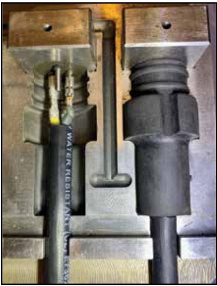
Two-pin plug with grounding bracket in a two-cavity mold.
