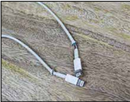
Figure 4. Solid strain relief gone bad! This method requires extra attention to work correctly
