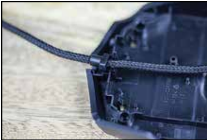
Figure 6. Slide-on designs, as seen in the Logitech mouse, are a low-cost alternative
