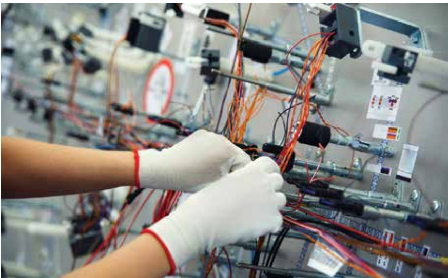
Figure 2: Wire harness manufacturing is still a labor-intensive process relying on manual assembly.
