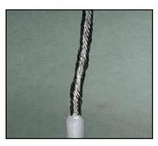
Figure 10. Overtwisted wire.
