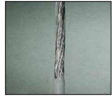
Figure 9. Birdcaging of straightened wire.
