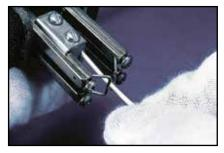
Figure 6. Firm insulation contact.
