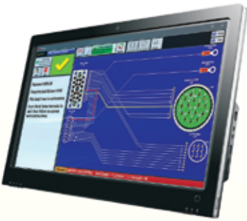
Production Continuity & HiPot Pass/Fail Check GUI
