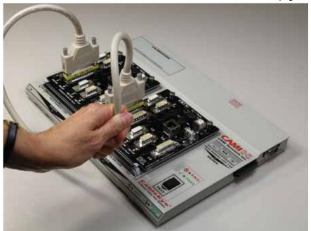
Figure 2. Intermittent Fault Check.
