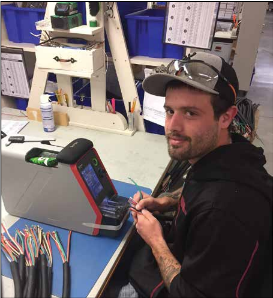
Billy strips wire for a multi-conductor assembly.
