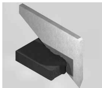
Example of a no-linear material such as rubber seizing onto a sliding shear at high speed.
