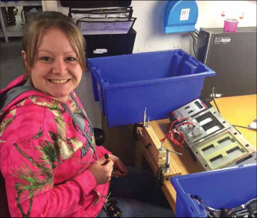
Meranda circuit testing an assembly.
