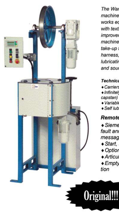
The Wardwell Harness Braider is the ideal machine for over braiding on harnesses. It works equally well with wire materials or with textile and synthetic threads. The improvements to this type of standard machine include: a motor driven capstan take-up for accurate coverage of the harness, a new tubular frame, a self lubricating horn gear, a new operator station and sound reduction, among many others.
