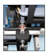
One-pulse wire splicing up to 100mm<sup>2</sup> and tinned wire to 60mm<sup>2</sup>. We've been using our patented Wedge-Reed System since 1960 to provide the most durable, precise welds of any ultrasonic metal welder manufacturer.
