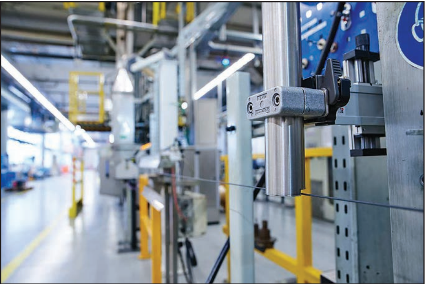
JET Rapid at work: 128,000 electrically charged ink drops fly towards the gutter every second.
