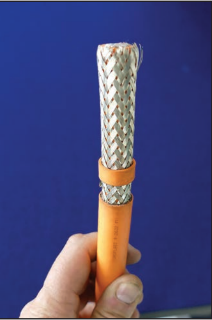
Laser strip on multi-layer cable wires inline from spool to spool using a precision wire transport system. With
