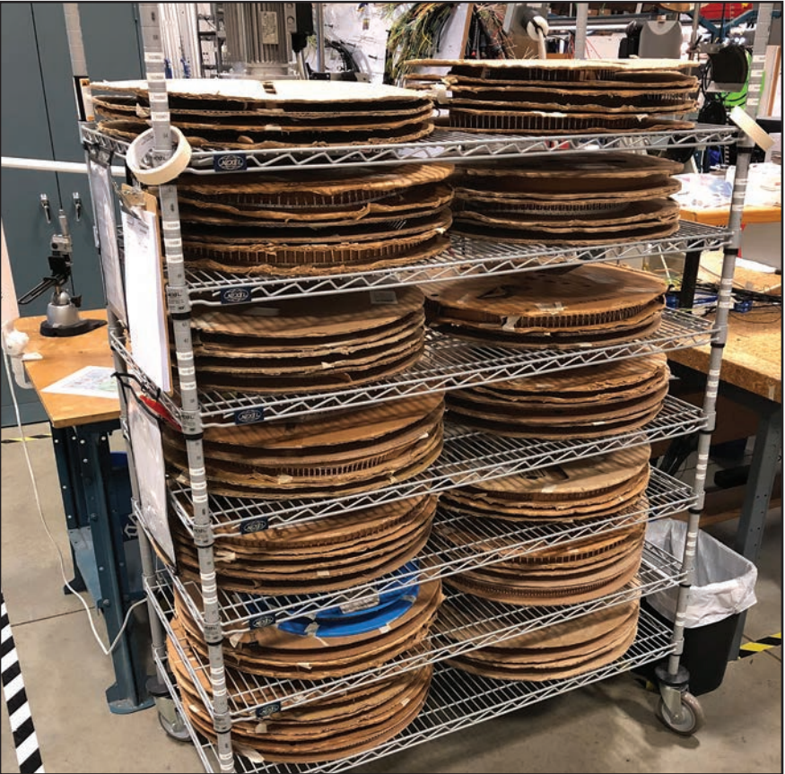
Figure 2. Proper reel storage on pie shelf
