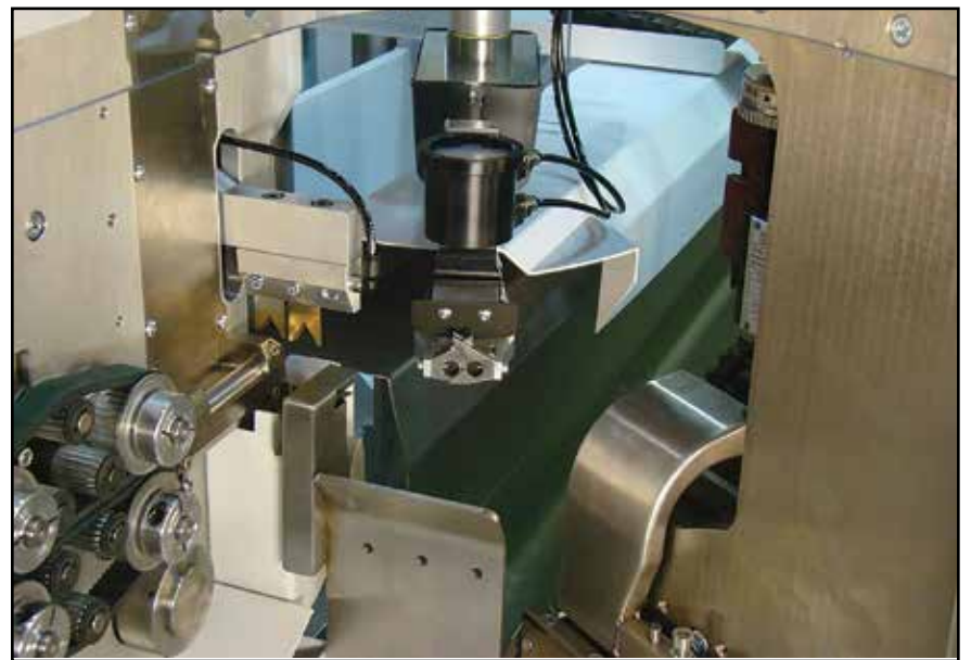
Figure 2. View of machine's servo cutterhead and swing arm.
