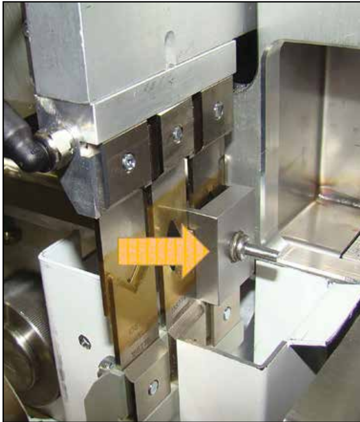
Figure 3. View of master setup fixture installed in blade-holder area prior to zero-point calibration.
