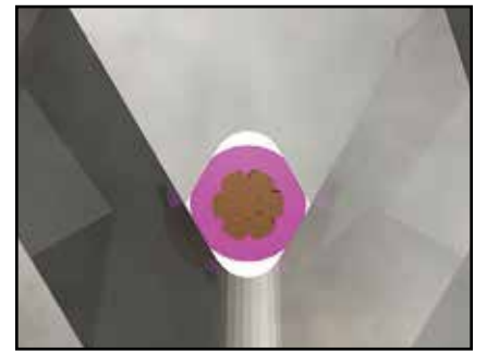
Figure 8. Depiction of a blade set which is not manufactured to calibration tolerance, the blade's relative opening to point zero calibration does not match the programmed gauge in the operator's setup screen menu.
