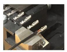
Figure 4. Placing a wire in the terminal
