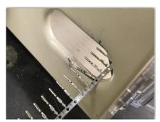
Figure 3. Terminal catching on a terminator guard
