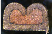
Figure 5. Flash on a 0.172mm crimp
