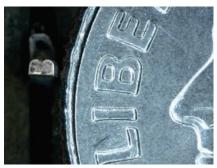
Figure 1. Comparing the size of a crimp with 0.17²mm wire cross sectional area to that of a U.S. dime
