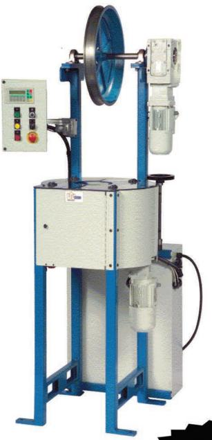
The Wardwell Harness Braider is the ideal machine for over braiding on harnesses. It works equally well with wire materials or with textile and synthetic threads. The improvements to this type of standard machine include: a motor driven capstan take-up for accurate coverage of the harness, a new tubular frame, a self lubricating horn gear, a new operator station and sound reduction, among many others.
