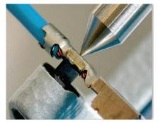
Figure 7. Crimp height inspection with micrometers
