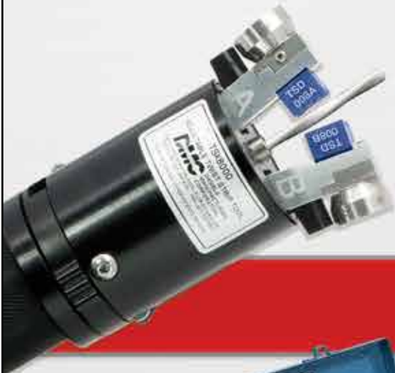
Tracks lay of oval cable for safe jacket removal
