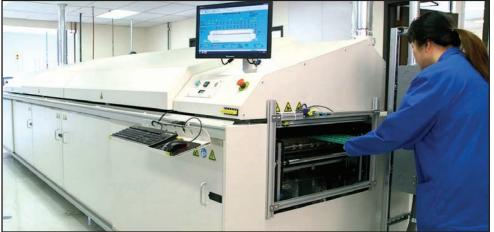
Adding nitrogen minimizes device failure and ensures printed circuit board integrity
