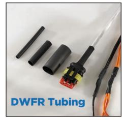
TE's DWFR tubing is applicable to a broad range of electrical connections and terminations. The product line comprises 14 sizes from 3 to 52mm (inside diameter). Of those, seven have 3:1 heat shrink ratios and seven have 4:1 ratios. The high shrink ratios can be particularly useful when applying this tubing to a connectorto-cable transition or to fit over a connector when making a cable jacket repair to an existing harness.
