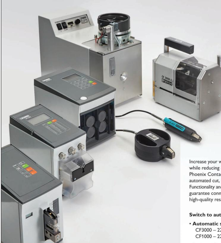
Increase your wire productivity, while reducing operator fatigue, with Phoenix Contact's bench-mounted, automated cut, strip, and crimp machines. Functionality and quick die-change capability guarantee connector adjustability and high-quality results.
