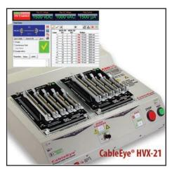
line. The HVX-21 extends the HiPot test voltage range to 2100 Vdc and 1200 Vac permitting detection of even more subtle defects.
