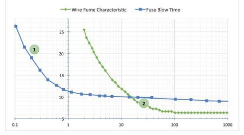
Figure 6: Fuse blow time and wire smoke time.
