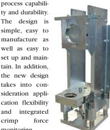
The frame is made of formed sheet metal rather than solid pieces of heavy steel or a cast frame, and instead of the conventional motor and gearbox combination, a direct belt-drive system is used. A patented ram spring mechanism is incorporated into the press ram, providing excel-
