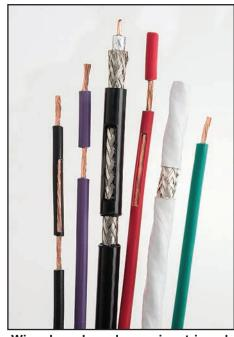
Wires have been laser wire stripped.
