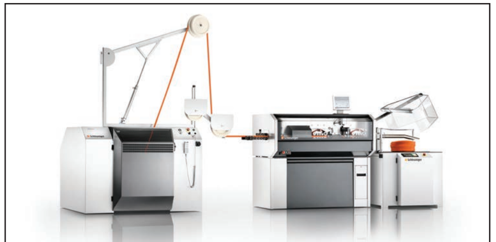
Schleuniger Prefeeder 4560, MegaStrip 9650, Cable Coiler 4000
