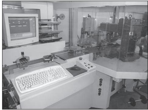
Lamcor's fully automated MTX machine crimps wires and has a crimp force monitor to assure quality control.
