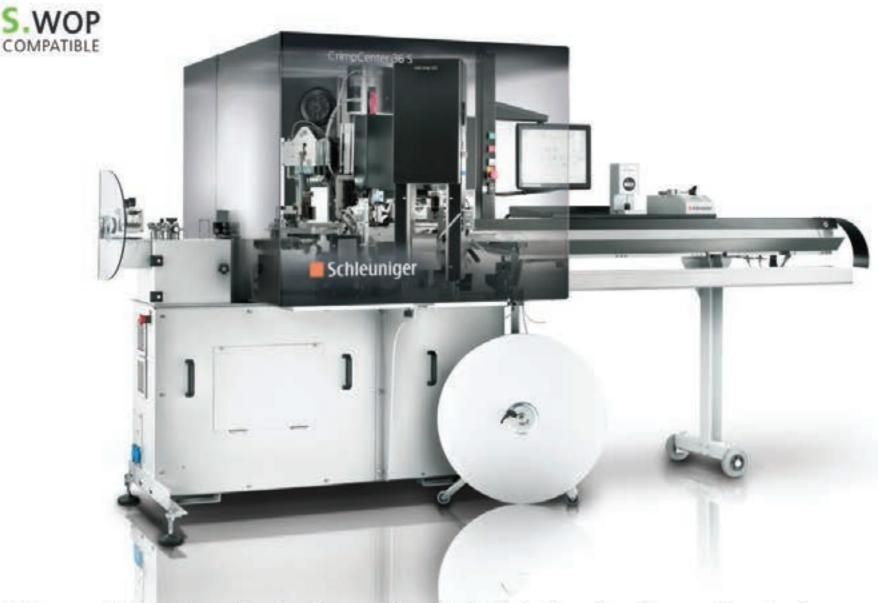
High speed fully automatic crimping machine that efficiently cuts, strips and terminates a wide range of wire types and sizes.
