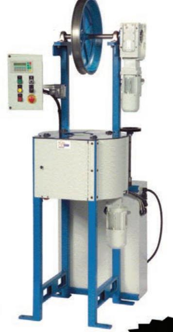
The Wardwell Harness Braider is the ideal machine for over braiding on harnesses. It works equally well with wire materials or with textile and synthetic threads. The improvements to this type of standard machine include: a motor driven capstan take-up for accurate coverage of the harness, a new tubular frame, a self lubricating horn gear, a new operator station and sound reduction, among many others.
