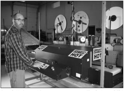
Data Cable invested in a new conveyor oven. Tim Cathcart, CI/QA Manager is working on the oven parameters for a new assembly using a conveyor oven purchased for their Military contracts.
