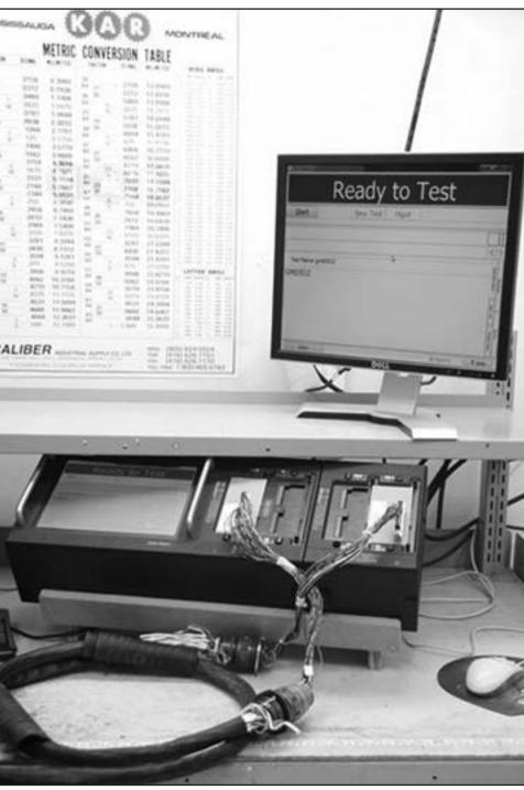
Basic fixturing to a Cirris Easy Touch provides in-process testing before the assemblies are "closed up".
