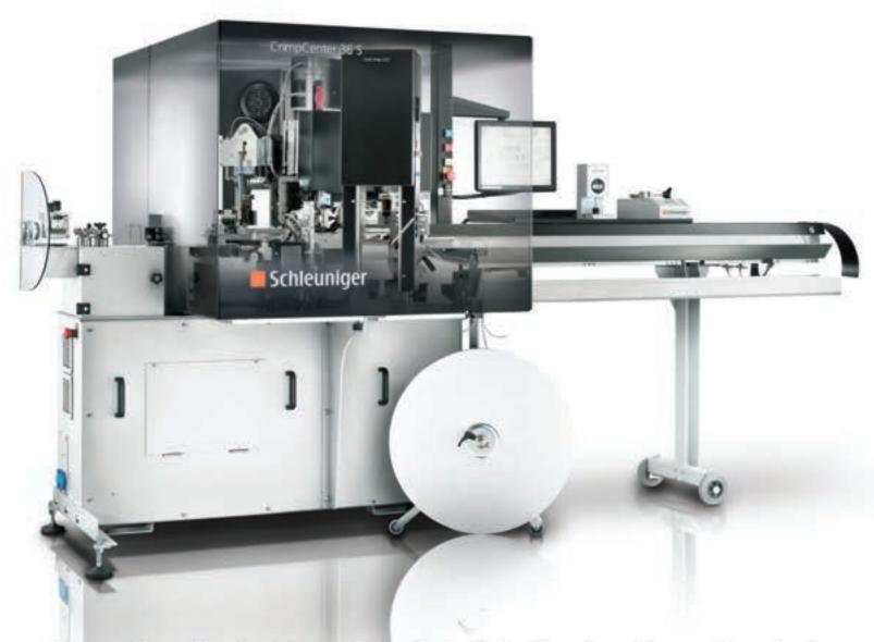
High speed fully automatic crimping machine that efficiently cuts, strips and terminates a wide range of wire types and sizes.
