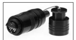
"Genderless" connectors have both male and female elements, and perhaps are more appropriately described as dual-gender. They are designed for quick deployment allowing the user to unreel fiber cable without regard for male or female ends.
