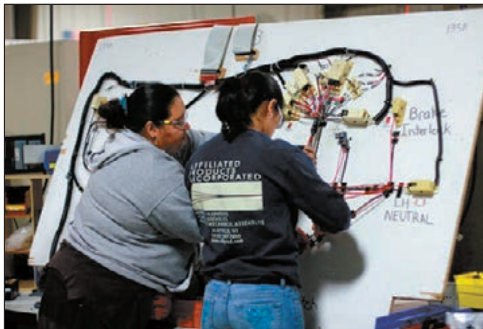
Erika Aguilar and Christina Meza of Affiliated Products fully assemble and 100% electrically test a wiring harness.
