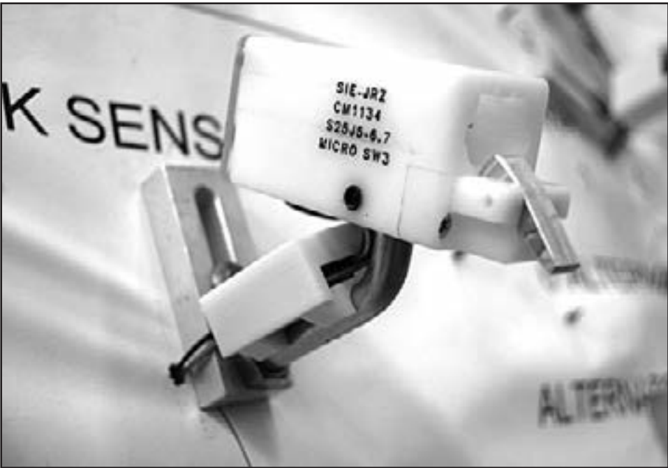
Fig. 1 - A BRAVA module retrofitted to the base of a typical holder.
