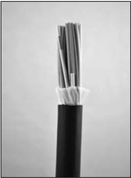
OCC's HC-Series high-density cables offer up to a twenty percent reduction in diameter and weight relative to conventional loose-tube cables, allowing for a greater fiber density and cable packing within ducts.
