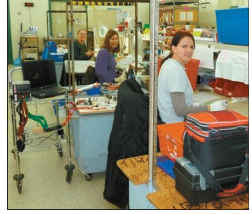
The NRI Data Cell assembling the less complex harnesses. All harnesses are tested using the Cirris Easy Tester on the cart.
