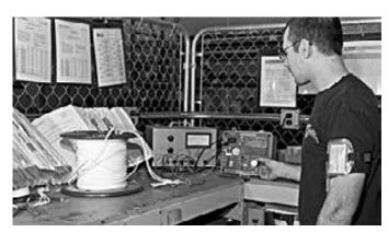
Allied Wire and Cable tests its cable in-house. Here, the cable undergoes hipot testing.
