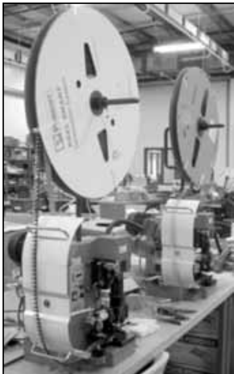
Bench top presses are used for low volume crimping.
