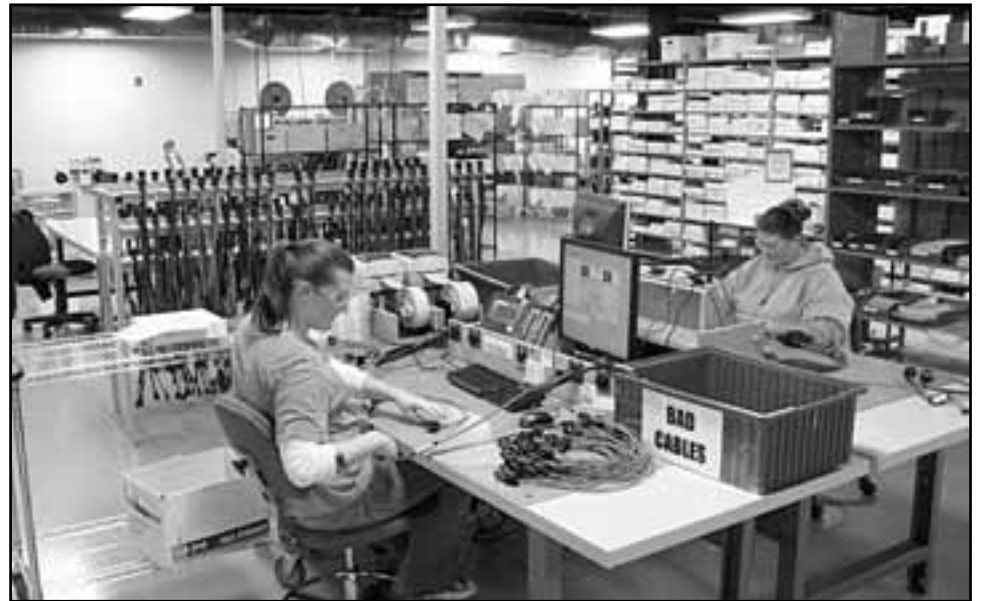
Custom made testing software works with the ERP system and a tester. Employees enter in the work order number the computer enters the test in the tester.
