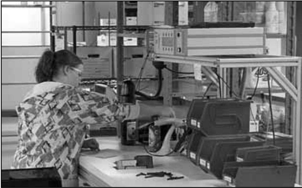
A one piece flow setup with a Stapla welder, and focus light help keep the product moving.
