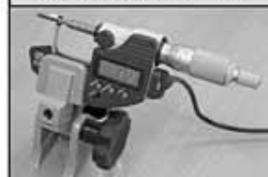
Measure conductor and insulation crimp heights
