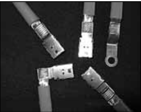
Typical Wire Termination Examples
