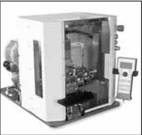
Figure 2: Typical Stripper Crimper for loose piece contacts.
