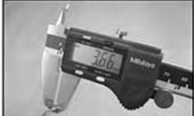
Measure conductor and insulation crimp widths
