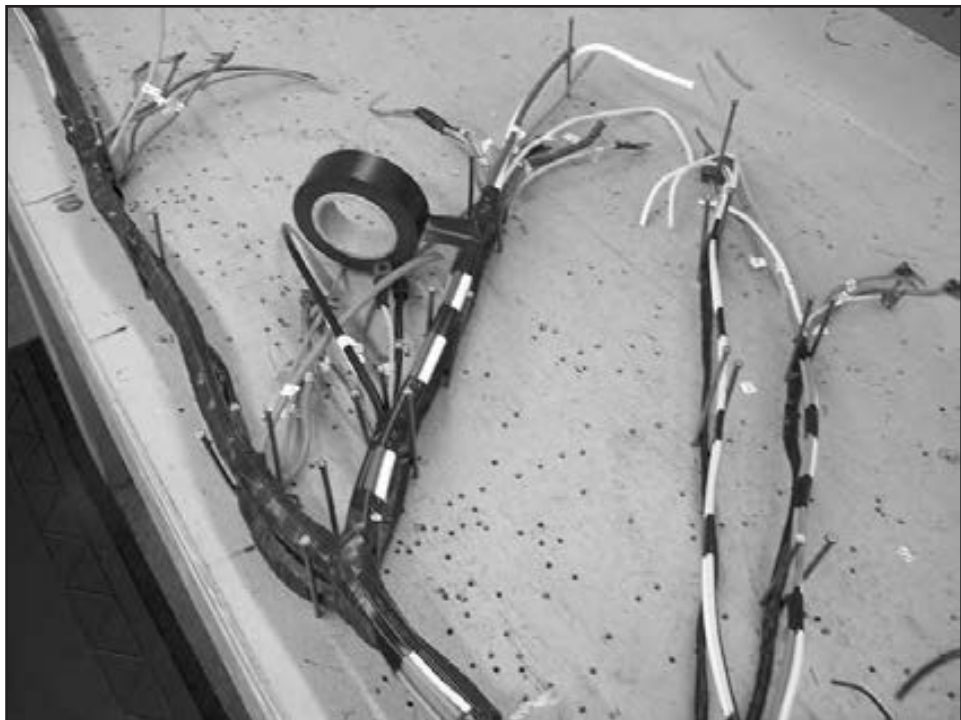
Some harnesses require the application of “old fashioned” rubber tape wrap as in the above harness.
