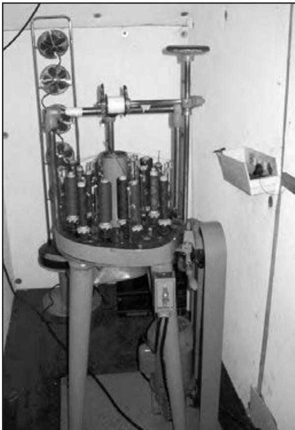
YnZ's uses a New England Butt 16-Carrier Braider for small diameter braiding jobs.
