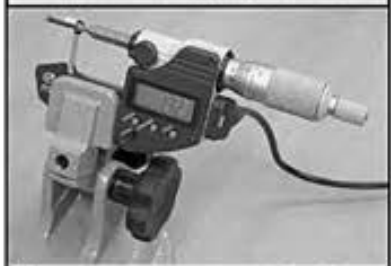
Measure conductor and insulation crimp heights
