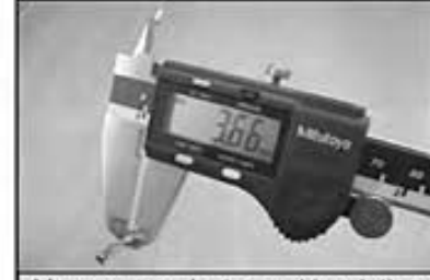
Measure conductor and insulation crimp widths
