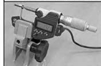
Measure conductor and insulation crimp heights
