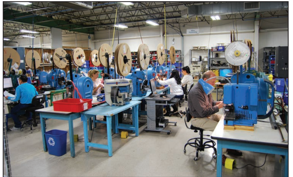
Fourstar Connections employees pinning wires on an extensive array of equipment.
