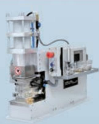
MANUAL module / Hot crimping / wire termination
