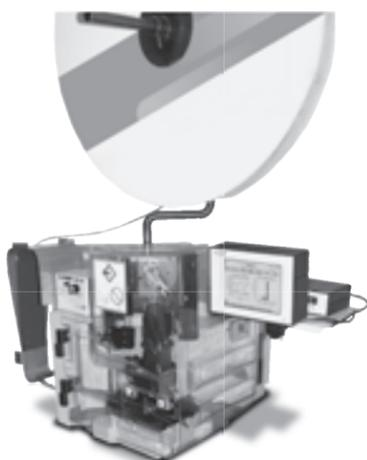
A wide range of optional equipment is available to meet your specific application requirements. By offering features such as tool-less precision crimp height adjust, a CQM II capability, batch counter and a work light as options, the AMP 3K/40 and AMP 5K/40 can be tailored to the specific application requirements without inflating the price for unwanted features.
